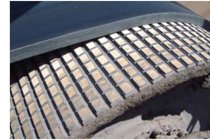
low-friction CERASINT lagging on tail pulley
