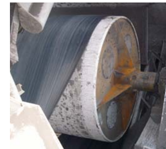
Drive pulley with high - friction CERADRIIVE NORUB lagging
